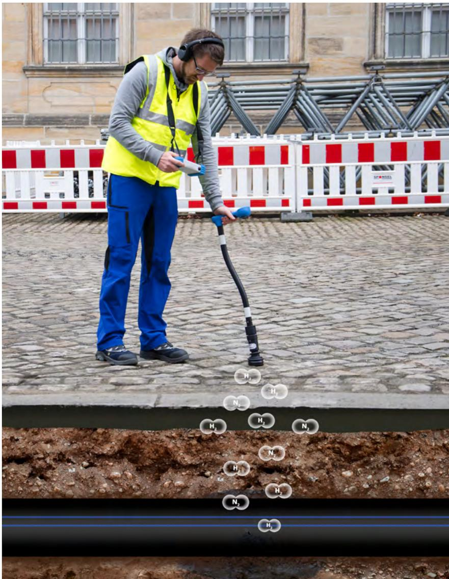
As well as the noise or trace gas sensor, you can also use the wired universal microphone. This can be directly connected to the HL 7000 operating unit. You can therefore conveniently “listen inside the pipe” in order to distinguish between leakage noise and potential interference.
