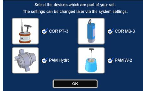
The statements made here determine which measuring methods will be offered in the Correlator's Start screen.
